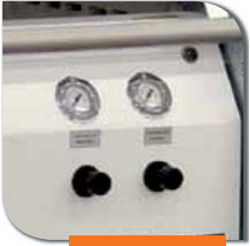
Two level assist gas Kit for cutting/marking
